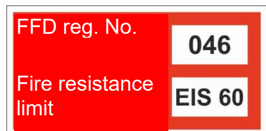
Figure 37 – sample designation of fire-fighting doors
