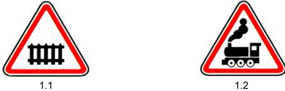
Figure 11 – signs 1.1 “Railroad crossing with bar gate” and 1.2 “Railroad crossing without bar gate”
