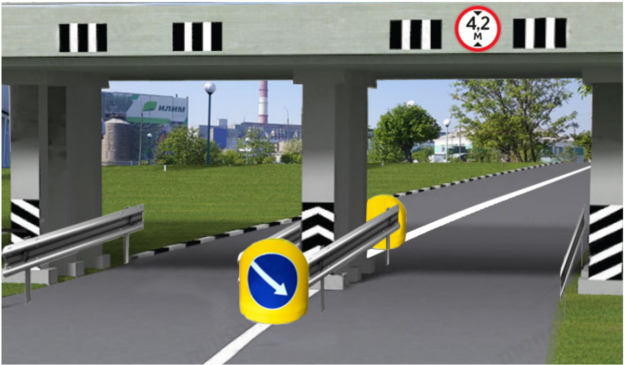
Figure 16 – samples marking on road structures
