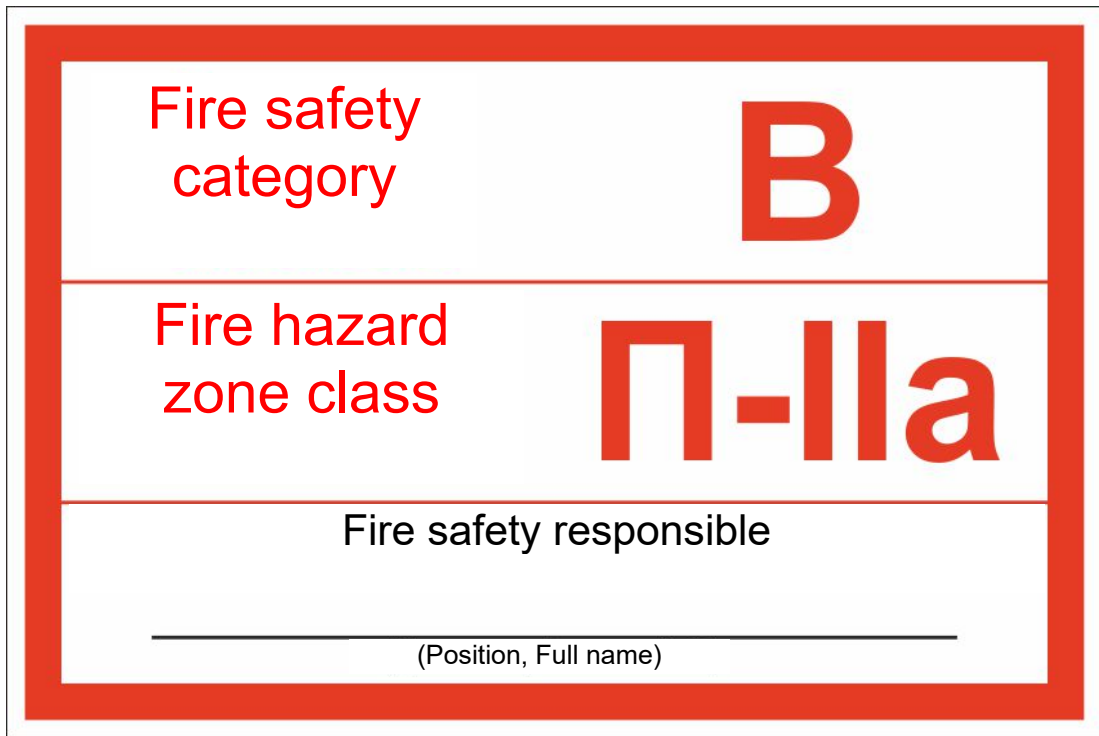
Figure 6 – sample plate for designation of explosion and fire hazard categories of buildings and rooms, fire hazard and explosion hazard class.
