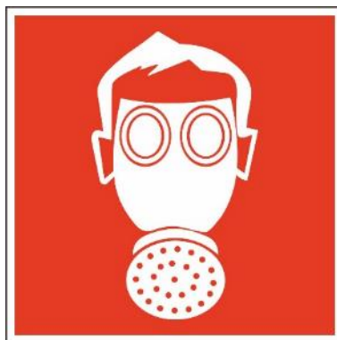
Figure 56 – sign F12 “Personal protective equipment location”
