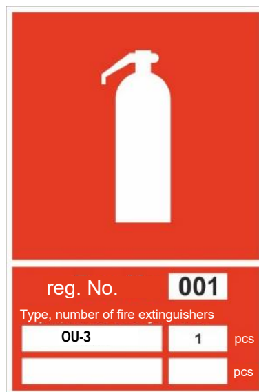
Figure 41 – sample of fire extinguisher location with an information plate
