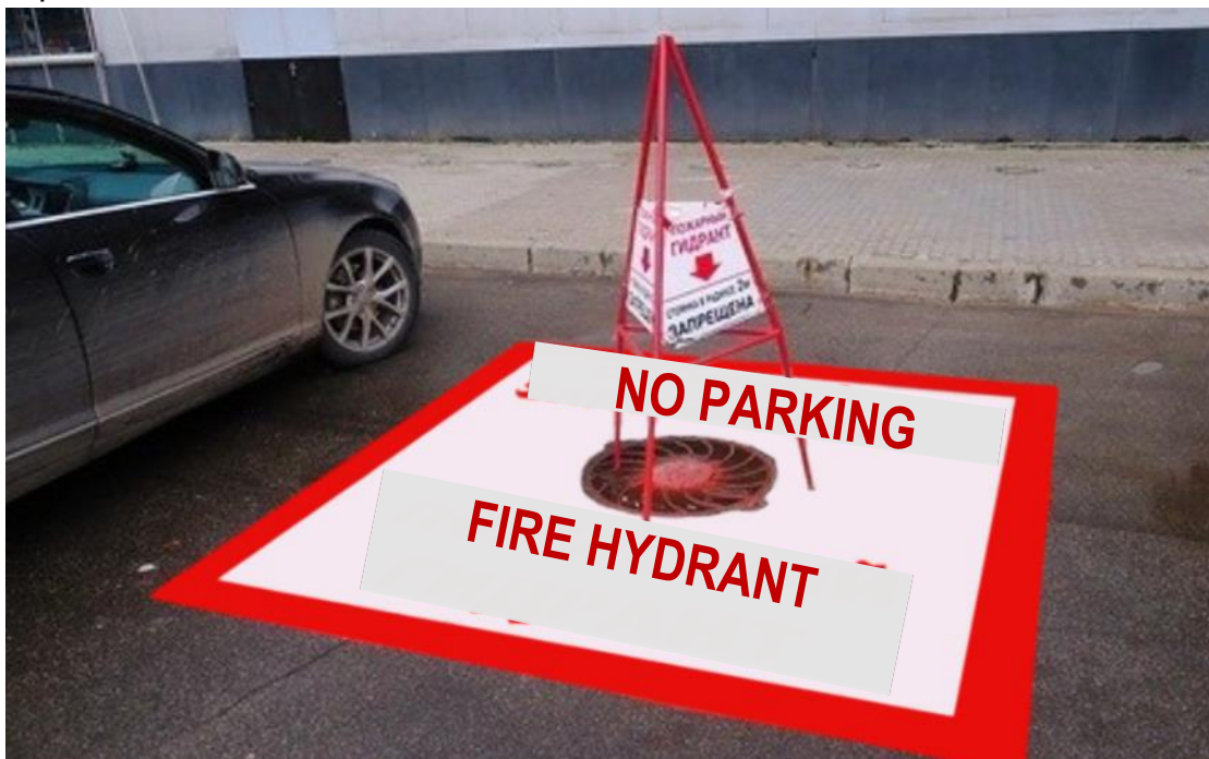
Figure 49 – sample designation of fire hydrant locations
